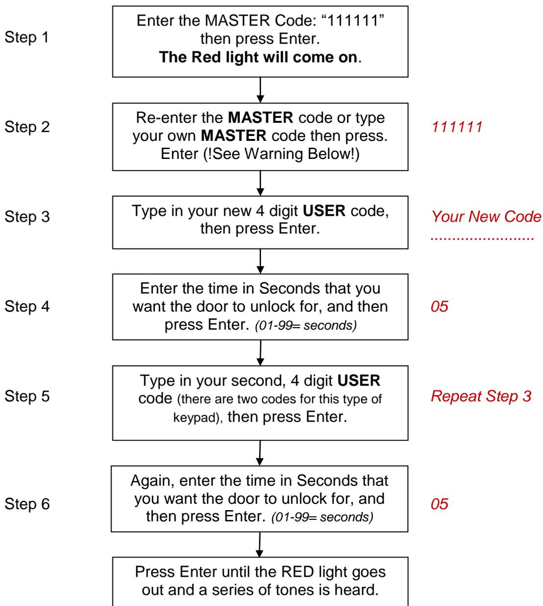
Typically, 5 seconds (05) in steps 4 & 6 is sufficient in time for the keypad to operate but if you need further guidance, please contact us for advice
